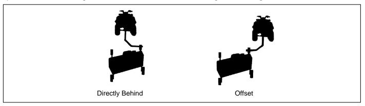
Figure 7: Rough Cut Tow Behind Towing Suggestions
